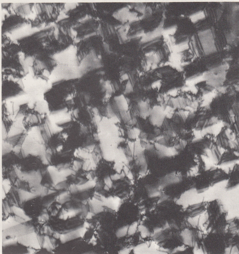
Fig. 10 Electron microscope photograph of typical single crystal gold film. 90,000X
